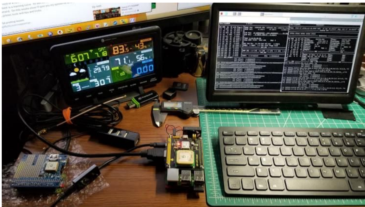
Pi0 on the left, Pi3 in the middle time servers running, gpsmon is visible for both of them. The color screen is a weather station, not related to this project. It also gets time from the network.
